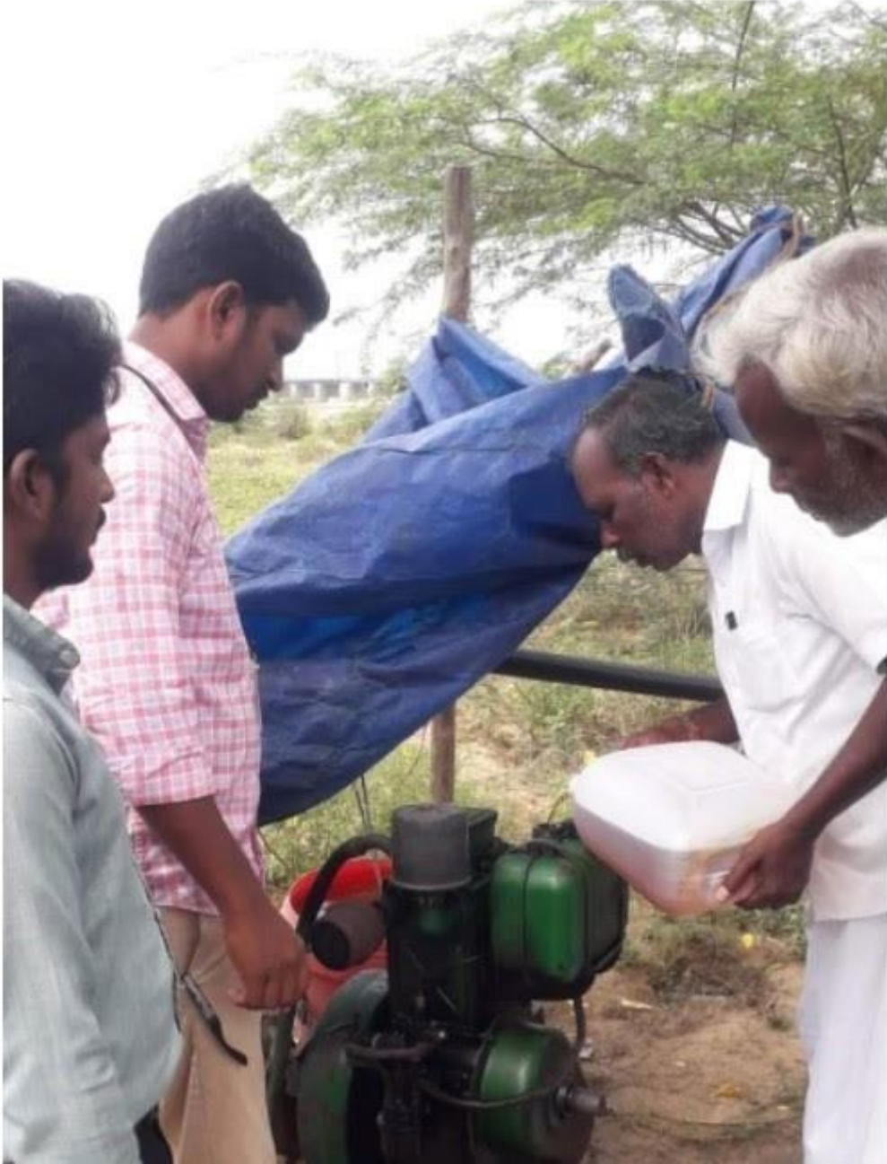
Pumpsets being fuelled with Biodiesel
