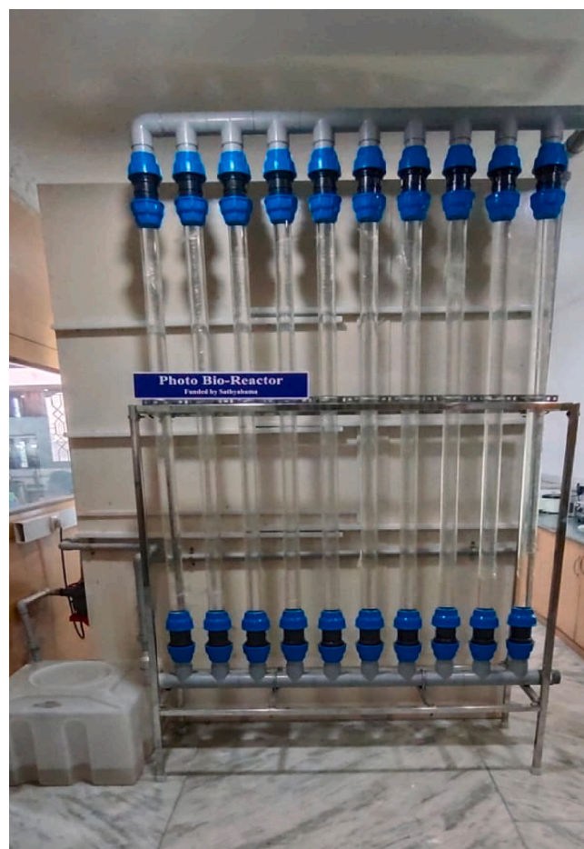
Fig. 3. Schematic representation of tubular photobioreactor for the indoor cultivation of microalgae.
